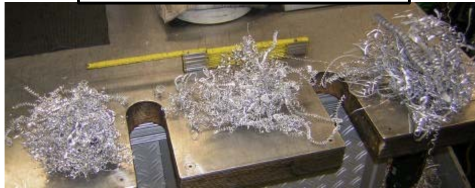
Long Curly Chips At Pump Inlet
