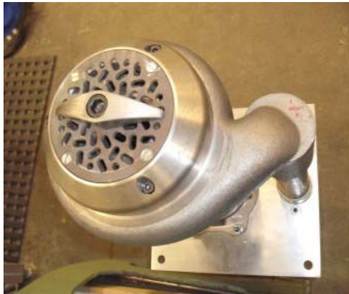
Tank installation pump with cutting tool
