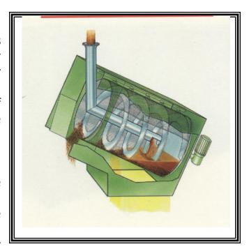
drum which helps transfer the return coolant laden with chips and swarf inside RolScreen Filter.
