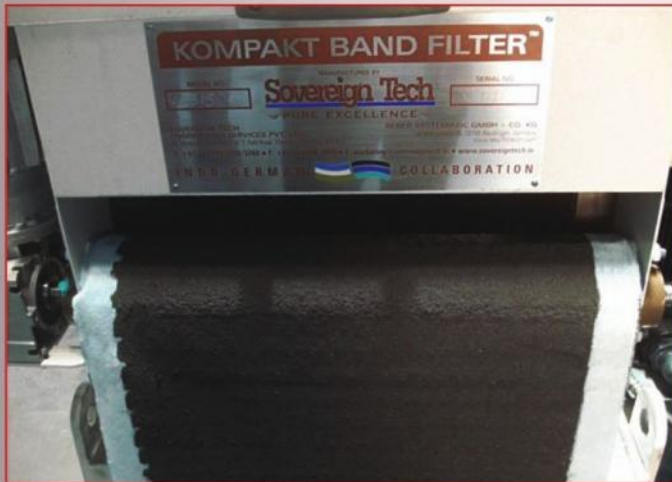
Arrest of Cast Iron fines and Graphite with perfect side sealing
