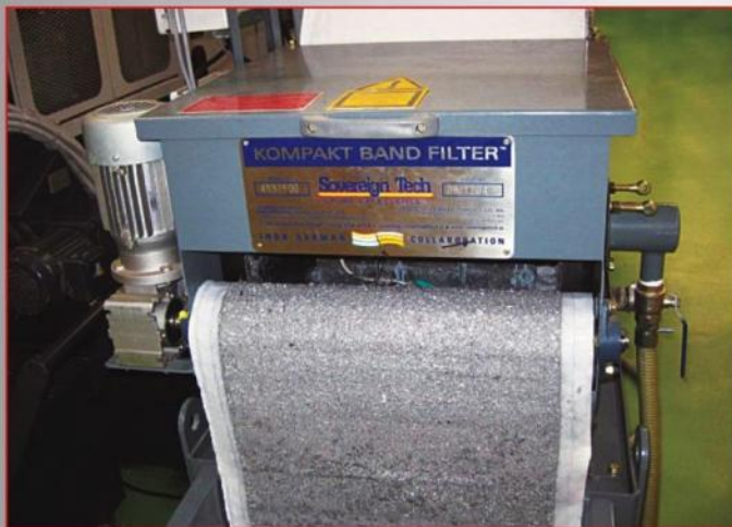
Arrest of Aluminum fines and Silica with perfect side sealing
